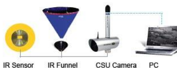
Figure 2: Diagram of the Akvasmart AQ1 Feeder system, showing method of deployment and flow chart for the feed management system (source: Akvasmart website, http://www.akvagroup.com ).
